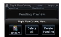
On the GTN device, while viewing the Flight Plan page, touch the **Menu** key and then the **Catalog** key to display the Flight Plan Catalog.
